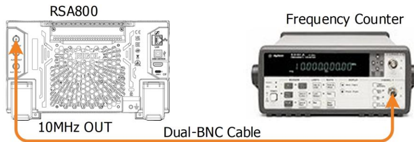
Figure 4.9 10 MHz Reference Output Accuracy Test Connection Diagram
