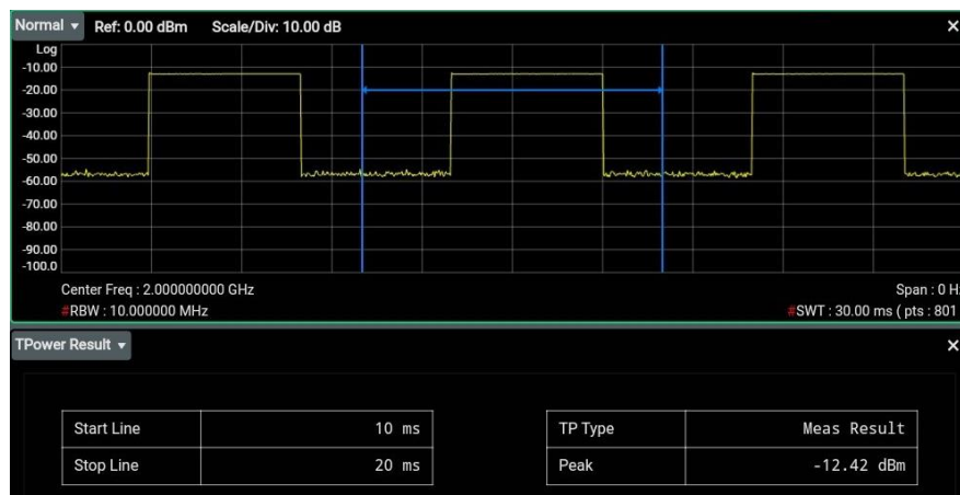
Figure 5.9 T-Power Measurement Interface
