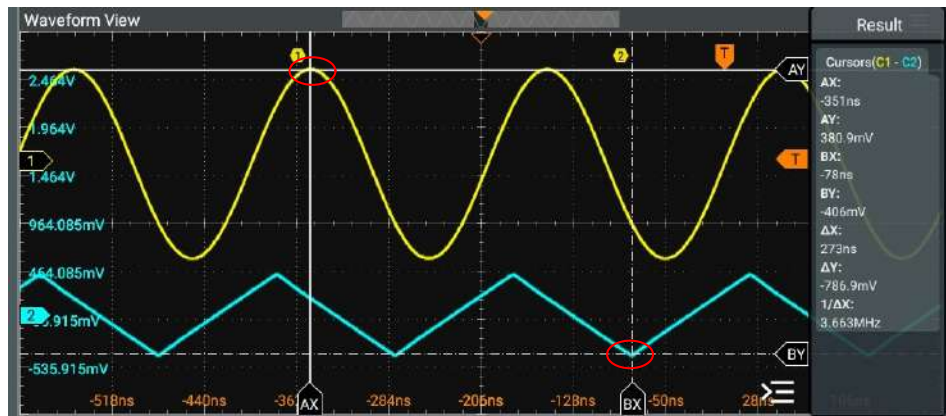
Figure 10.13 Track Measurement (after Horizontal Expansion)
