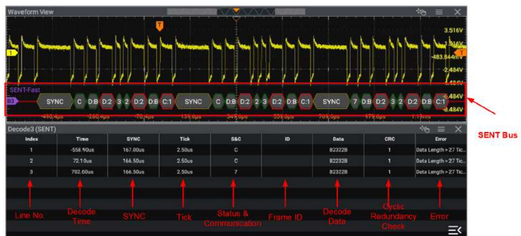
Figure 21.27 SSENT Decoding Event Table
