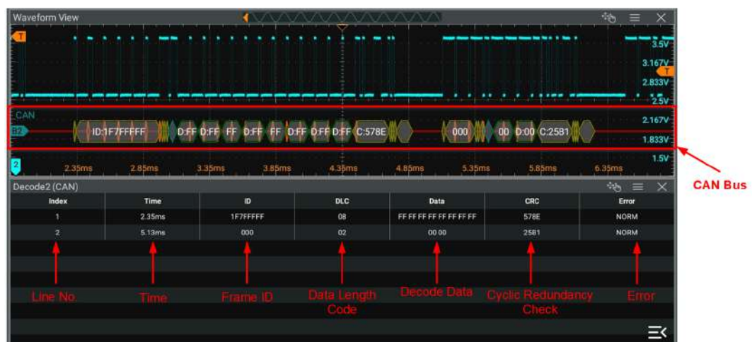
Figure 21.15 CAN Decoding Event Table
