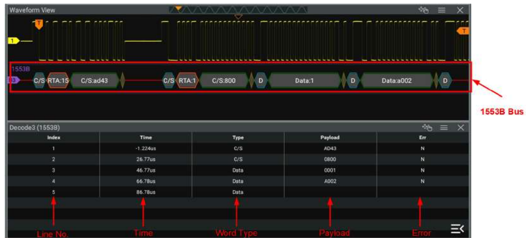
Figure 21.24 1553B Decoding Event Table
