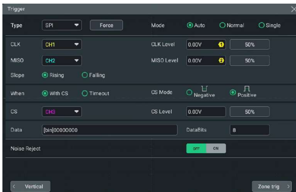
Figure 8.31 SPI Trigger Setting Menu
