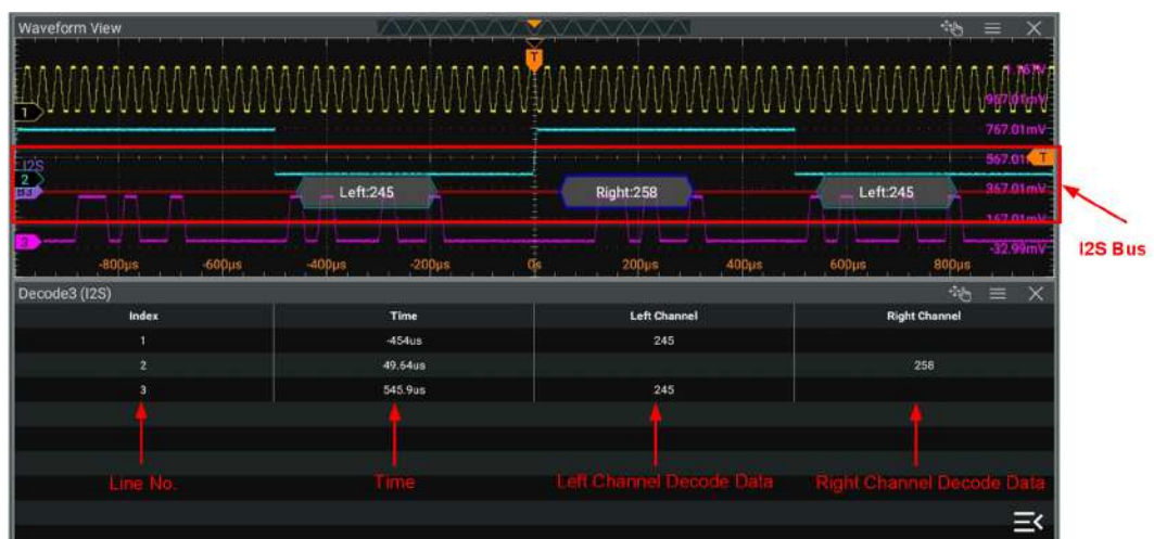
Figure 21.19 I2S Decoding Event Table
