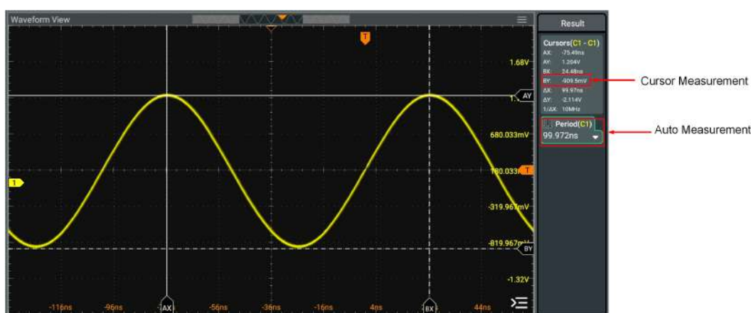
Figure 10.8 Manual Cursor Measurement Example
