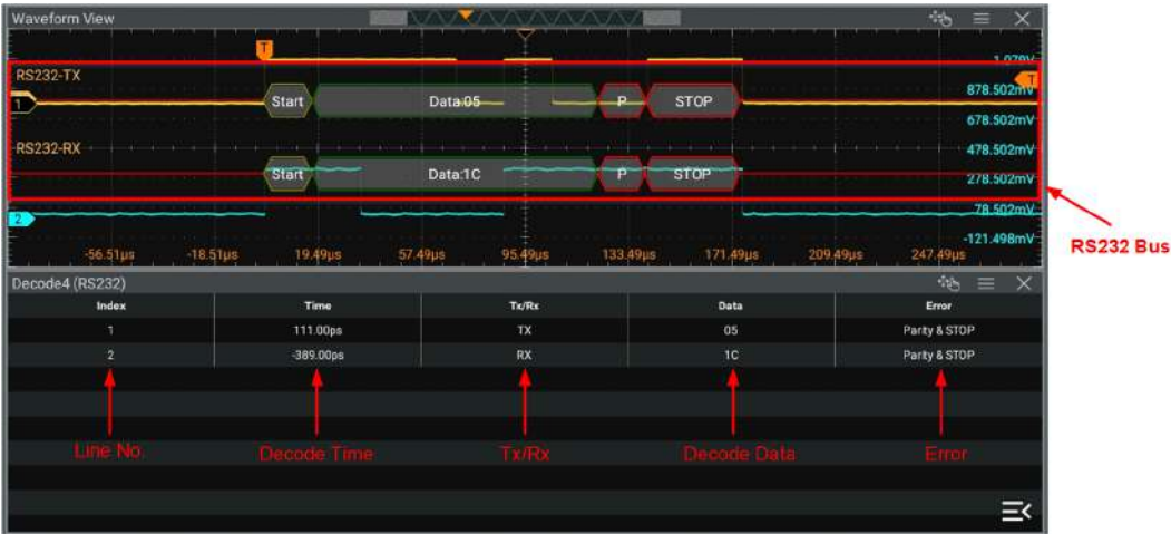
Figure 21.6 RS232 Decoding Event Table
