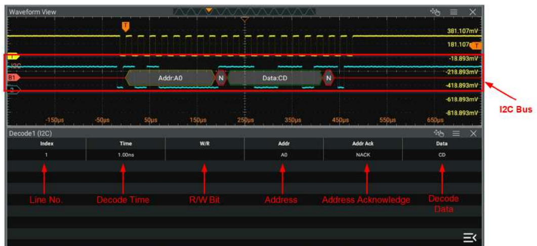
Figure 21.9 I2C Decoding Event Table
