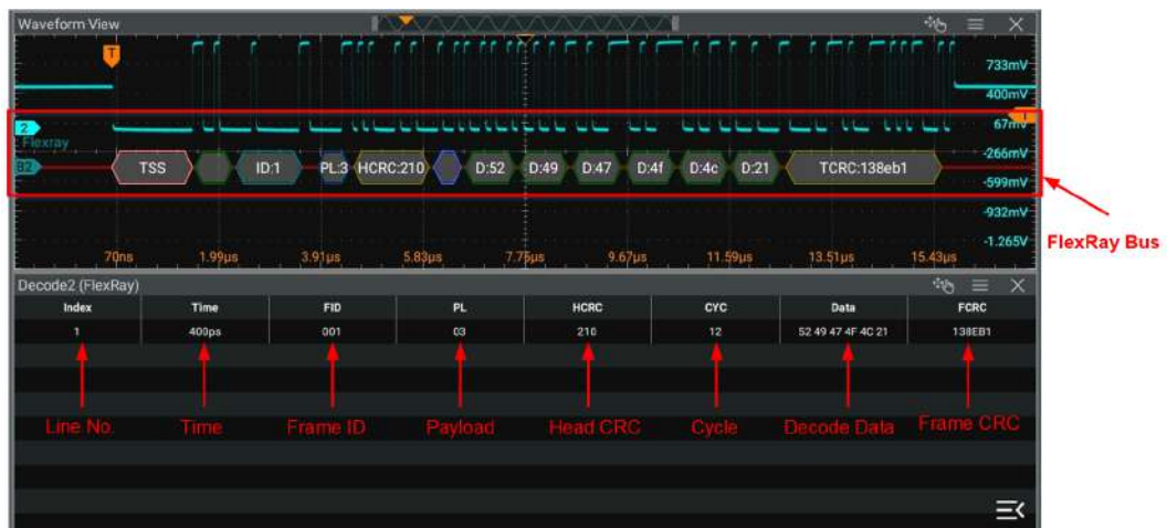
Figure 21.22 FlexRay Decoding Event Table
