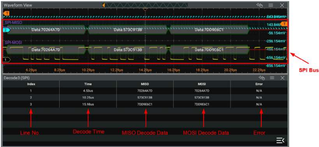
Figure 21.12 SPI Decoding Event Table
