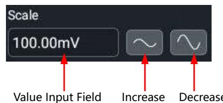
In the **Vertical** system menu, select **ON** or **OFF** to enable or disable the fine adjustment. By default, it is OFF. You can also press down the vertical scale knob on the small screen to enable or disable the fine adjustment.
