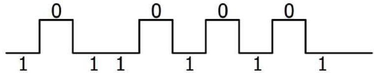
Figure 17.5 Schematic Diagram of Negative Logic
