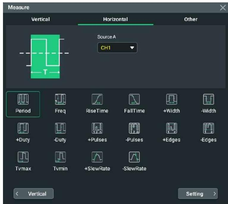
Figure 10.5 Horizontal Measurement Items
