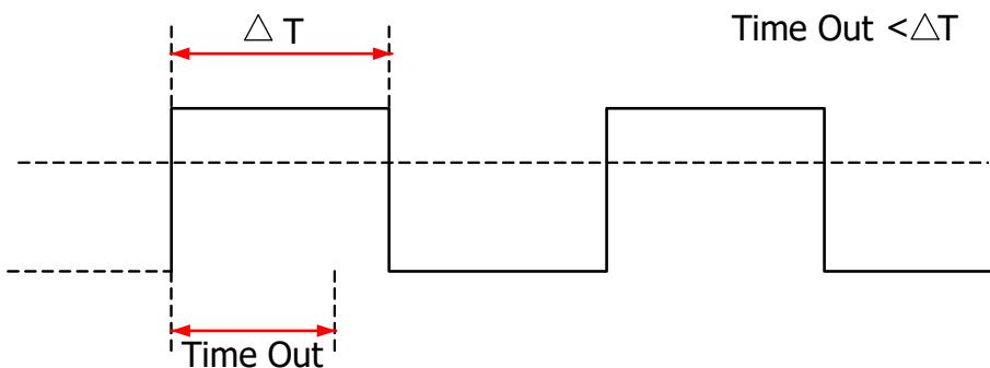
Figure 8.13 Timeout Trigger
