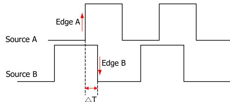
Figure 8.18 Delay Trigger
