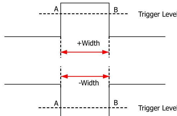
**Figure 8.4 Positive Pulse Width/Negative Pulse Width**
