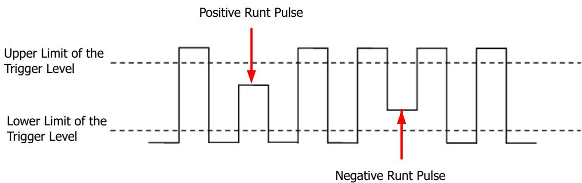
Figure 8.15 Runt Trigger
