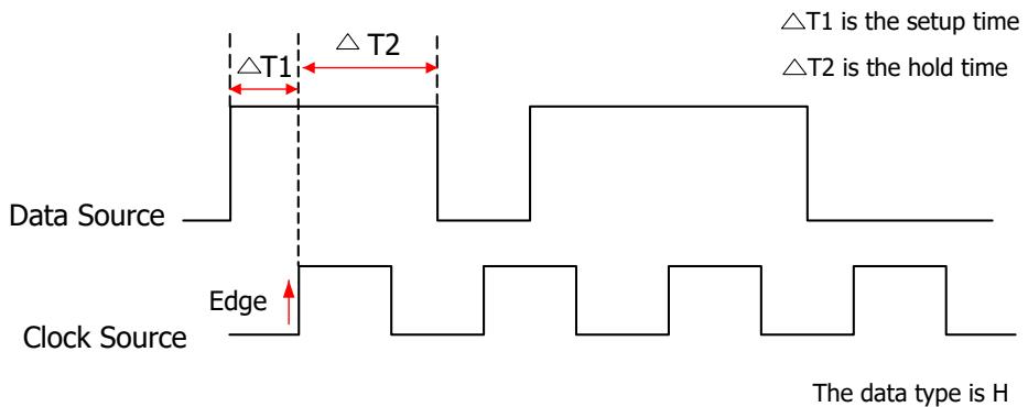
Figure 8.20 Setup/Hold Trigger
