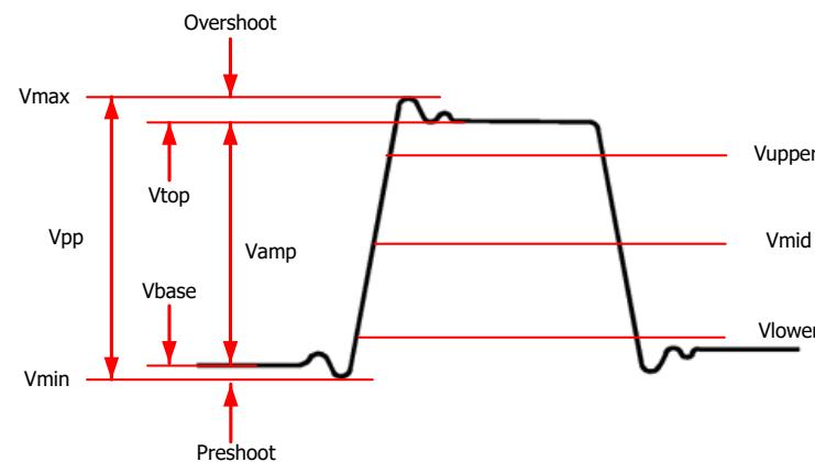
Figure 10.3 Voltage Parameters
