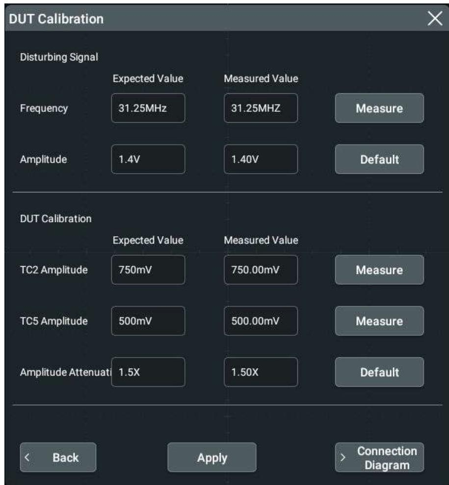
**Figure 18.8 Fixture Calibration**
