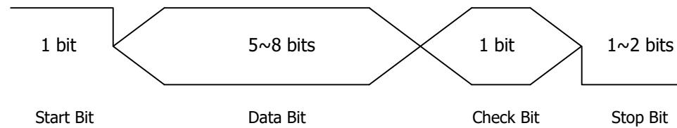
Figure 8.24 Schematic Diagram of RS232 Protocol
