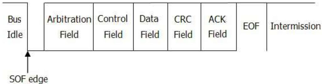
Figure 8.32 Data Frame Format of the CAN Bus
