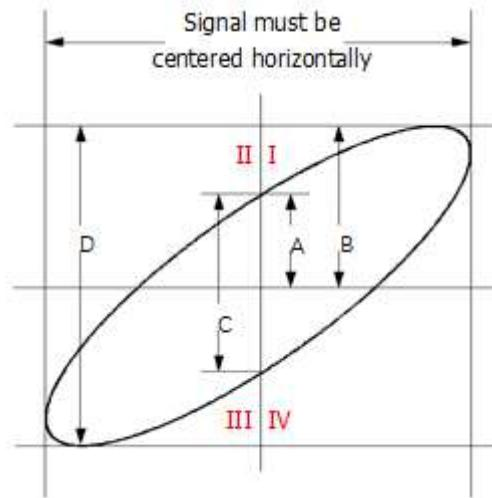
**Figure 7.3 Measurement Schematic Diagram of Phase Deviation**
