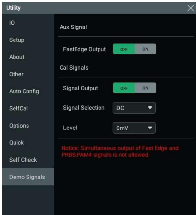
**Figure 24.7 Demonstration Signals Menu**
