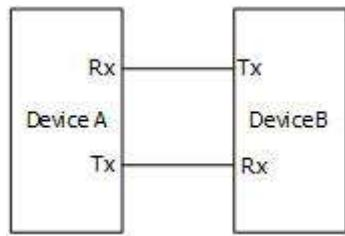
Figure 17.4 Schematic Diagram of UART/RS232 Serial Bus
