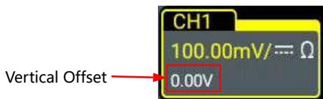
The adjustable range of the vertical offset is related to the current input impedance, probe ratio, and vertical scale.
