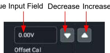
The range of bias is related to the input impedance and the vertical scale.
