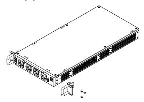
3. Use two M4x8 torx pan head screws to fasten the handle to the front bezel.
