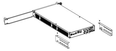
6. Mount the assembled instrument and rack into a standard 19-inch cabinet by using four M6x16 phillips pan head screws and four M6 square lock cage nuts.
