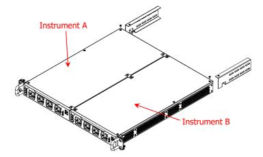
5. Mount the assembled instrument and rack into a standard 19-inch cabinet by using four M6x16 phillips pan head screws and four M6 square lock cage nuts.
