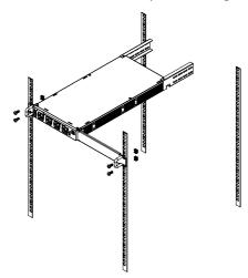
7. Use two M6x16 phillips pan head screws and two M6 square lock cage nuts to secure the rear hanging ear to the cabinet. Then use four M4x8 phillips pan head screws to secure the left side beam to the rear hanging ear.
