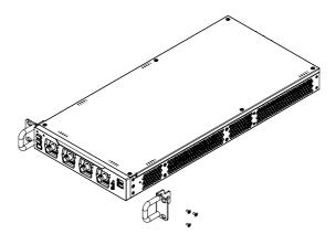
3. Using four connecting plates to fasten the two instruments with eight existing M3x6 torx flat head countersunk screws on the instrument.
