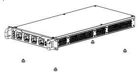
2. Remove six M3x6 torx flat head countersunk screws that secure the two hanging ears at a different side of each instrument. You only need to remove the hanging ear at one side for each instrument and keep the hanging ear at the other side unremoved.
