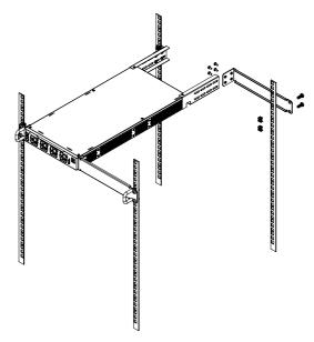
9. The following figure shows the front view of the successful rack mount installation for one instrument.
