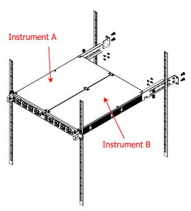
7. The following figure shows the front view of the successful rack mount installation for two instruments.
