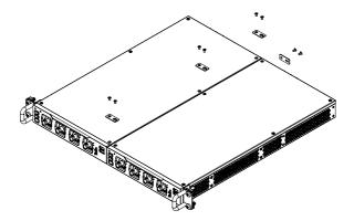
4. Secure the left side beam to the left side of the rear panel of Instrument A; and secure the right side beam to the right side of the rear panel of Instrument B by using the existing M3x6 torx flat head countersunk screws on the instrument.
