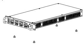
2. Remove three M3x6 torx flat head countersunk screws that secure the hanging ear of the instrument at the right side of the front panel. Then remove two M4x8 torx pan head screws that secure the handle. You only need to remove the hanging ear at one side and keep the hanging ear at the other side unremoved.
