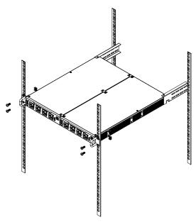
6. Use four M6x16 phillips pan head screws and four M6 square lock cage nuts to secure the two rear hanging ears to the rack. Then use four M4x8 phillips pan head screws to secure the left side beam of Instrument A to the rear hanging ear; use four M4x8 phillips pan head screws to secure the right side beam of Instrument B to another rear hanging ear.
