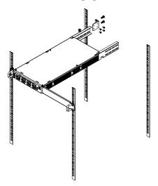
8. Use two M6x16 phillips pan head screws and two M6 square lock cage nuts to secure the rear bezel to the rack. Then use four M4x8 phillips pan head screws to secure the right side beam to the rear bezel.
