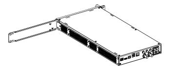
5. Secure the left and right side beams to the two sides of the rear panel by using the available M3x6 torx flat head countersunk screws on the instrument.
