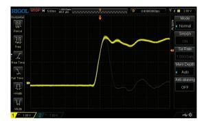
UltraVision: waveform recording and playback functions
